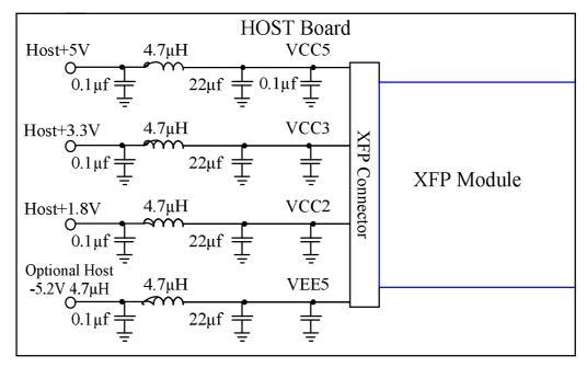
**Recommended High-speed Interface Circuit**
