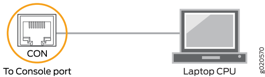
Figure 43: Connecting the MX204 Router Directly to a Management Console
