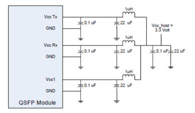
Figure 4. Recommended Host Board Power Supply Filter Network
