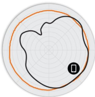
Figure 3. R610 5GHz Azimuth Antenna Patterns
