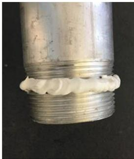
4. Thread NPT-NPS aluminum adapter coupling on the threaded end of the camera mount. Pay special attention to ensure the NPT threads are going toward the camera mount and the NPS end is going to the camera.
