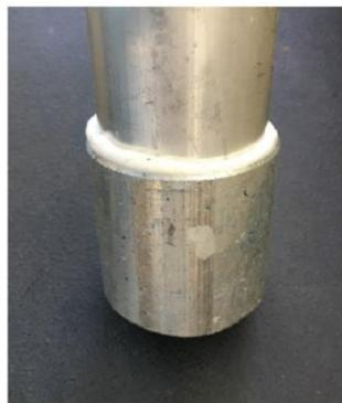
The adhesive sealant should be tack-free in 50 – 60 minutes with a full cure occurring at approximately 24 hours. There is no need to wait for the product to become tack-free before
