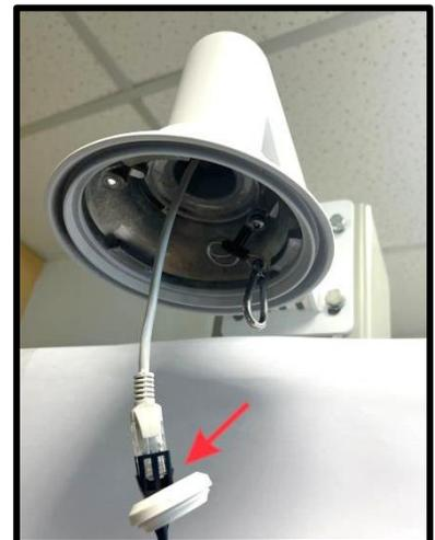
**NOTE:** Please thread the Ethernet cable straight through the grommet. Do not bend the Ethernet cable as it may cause damage to the grommet.
