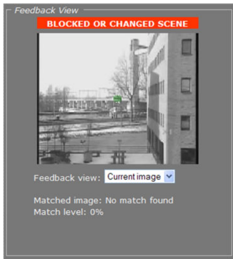
Camera has moved further to the right. Current image no longer matches any reference image, resulting in a changed scene alarm.
