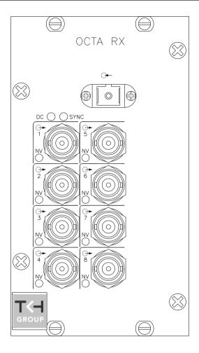
Figure 1. OCTA 40x0 RX front panel. TX panels look similar, with video inputs instead of outputs. See Table 1.
