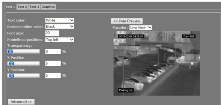
Video > OSD > Text 1, with three OSD bars in the preview (render modes: Border)
