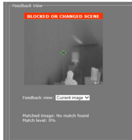
Camera lens is being spray-painted, resulting in a blocked scene alarm.
