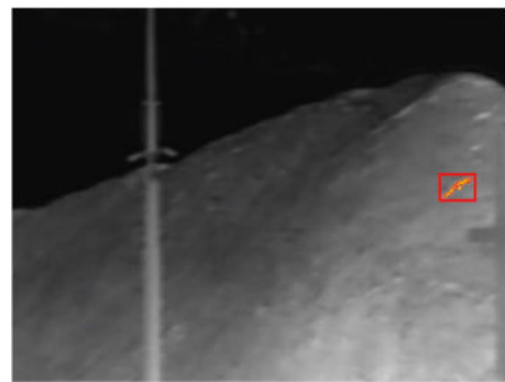
Smouldering detection (coal pile)
